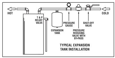
Expansion tanks are pre-charged with a 40 PSI air charge. If the inlet water pressure is higher than 40 PSI, the expansion tank's air pressure must be adjusted to match that pressure but must not be higher than 80 PSI.
