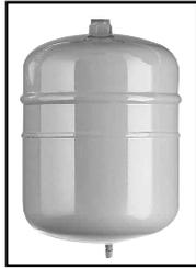
A properly sized U.S. Craftmaster Expansion Tank eliminates these problems, by giving water a place to go when thermal expansion occurs. When a water heating cycle ends, or when any fixture is opened within the system, the impact of thermal expansion is reduced, and water drains out of the expansion tank back into the system.
